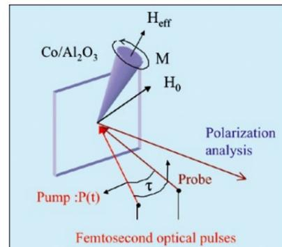
Fig. 1: Time resolved magnetization dynamics using femtosecond optical pulses.
