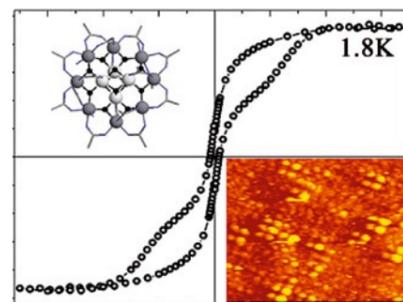
SQUID hysteresis of the monolayer  $Mn_{12}Piv_{16}$  showing a hysteresis loop, which is reminiscent of an assembly of single molecules. The first inset shows a schematic view of the  $Mn_{12}Piv_{16}$  molecule. The second inset shows an STM image of the self-organized molecular layer on Au(111).
