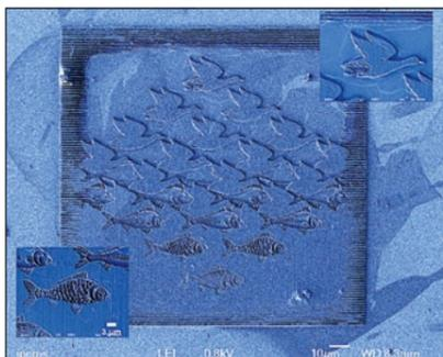
Nanopicture obtained by RBnano maskless engraving process (based on Escher original).
