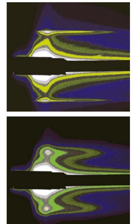
GISAXS signal of a Co deposit on Au(111) for two different crystallographic directions. The top picture reveals crystalline-type order whereas the bottom one shows liquid-type order.
