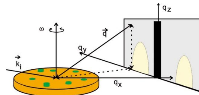
X-rays impinge on the surface with an incidence close to the total reflexion angle. The scattered intensity is recorded with a CCD camera, placed 1 meter from the sample. A tungsten beamstop (black rectangle) hides the specular beam.
