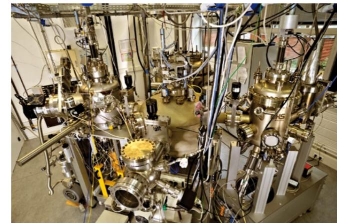
Experimental setup for the fabrication of tunnel junction multilayers.
