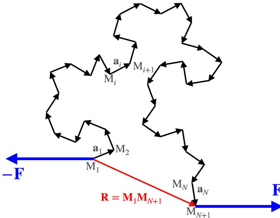
Figure 1: Sketch of a polymer chain (represented in 2d for simplicity) subject to external forces  $\mathbf{F}$  applied at its two ends, and composed of  $N$  monomers  $\mathbf{a}_i = \mathbf{M}_i \mathbf{M}_{i+1}$ , with  $|\mathbf{a}_i| = a$ . The end-to-end vector  $\mathbf{R} = \mathbf{M}_1 \mathbf{M}_{N+1}$  is shown in red.
