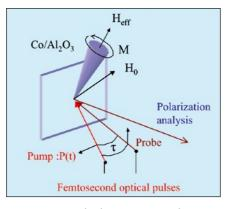
Fig. 1 : Time resolved magnetization dynamics using femtosecond optical pulses.
