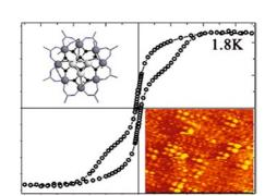
SQUID hysteresis of the monolayer Mn<sub>12</sub>Piv<sub>16</sub> showing a hysteresis loop, which is reminiscent of an assembly of single molecules. The first inset shows a schematic view of the Mn<sub>12</sub>Piv<sub>16</sub> molecule. The second inset shows an STM image of the self-organized molecular layer on Au(111).
