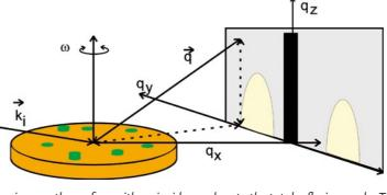
X-rays impinge on the surface with an incidence close to the total reflexion angle. The scattered intensity is recorded with a CCD camera, placed 1 meter from the sample. A tungsten beamstop (black rectangle) hides the specular beam.
