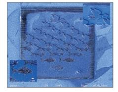
Nanopicture obtained by RBnano maskless engraving process (based on Escher original).
