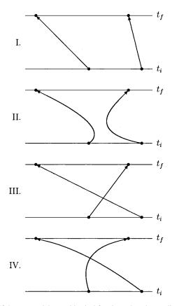
Fig. 1. If the two particles are identical fermions, then the amplitudes associated with interchanging paths, such as III and IV, must be multiplied by -1 before summing.
