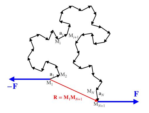
Figure 1: Sketch of a polymer chain (represented in 2d for simplicity) subject to external forces F applied at its two ends, and composed of N monomers  $a_i = M_i M_{i+1}$ , with  $|a_i| = a$ . The end-to-end vector  $\mathbf{R} = M_1 M_{N+1}$  is shown in red.
